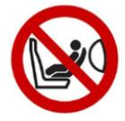
f) The AIRBAG OFF pictogram must be based upon that detailed in ECE R121 as shown below:
