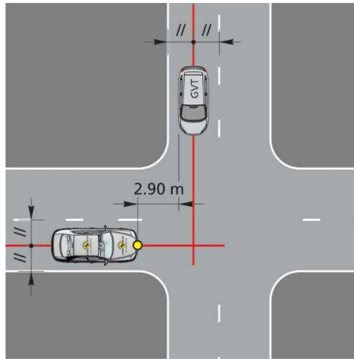
**Figure 8-9 SCP start from stop setup**
