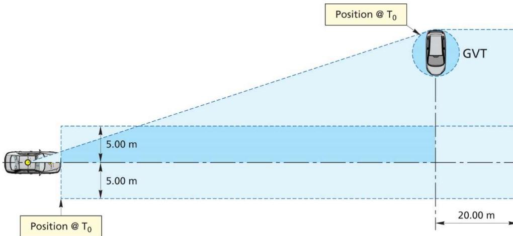
**Figure 7-3: Free space requirements – CCC Farside Test**
