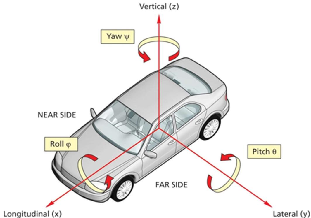
Figure 3-1: Coordinate system and notation
