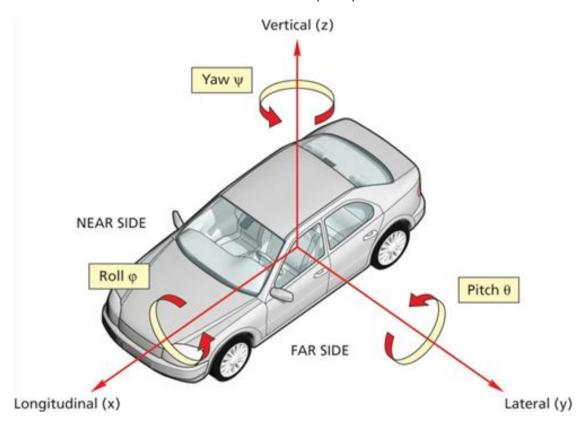
Figure 3-1: Coordinate system and notation
