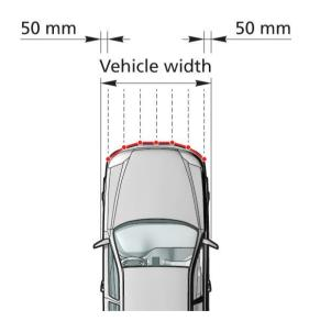
Figure 3-4 VUT Front bumper profile
