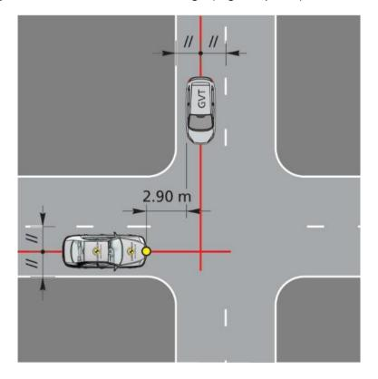
Figure 8-9 SCP start from stop setup
