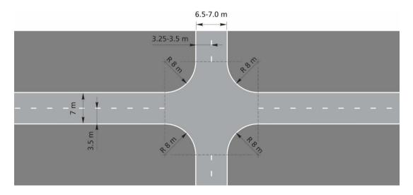
Figure 7-1: Layout of junction and the connecting lanes
