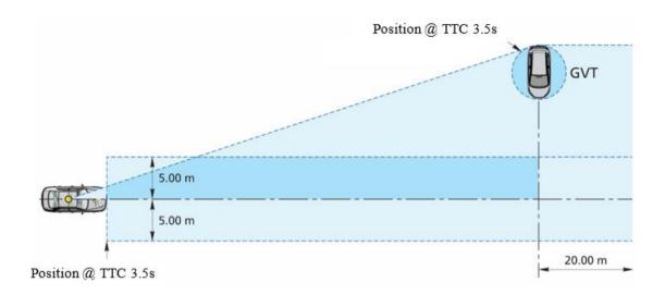
Figure 7-3: Free space requirements – CCC Farside Test
