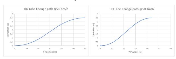
Figure 8-12 CCFhol path at 70 and 50 km/h
