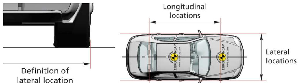
**Figure 6-5: Vehicle dimensional measurements**
