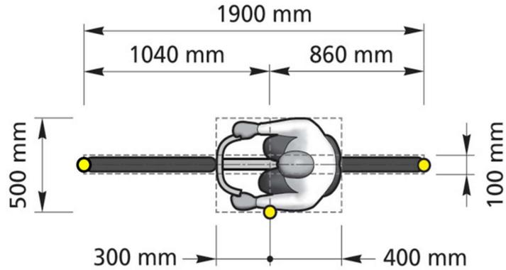
**Figure 3-5: Virtual box dimensions around EBT**
