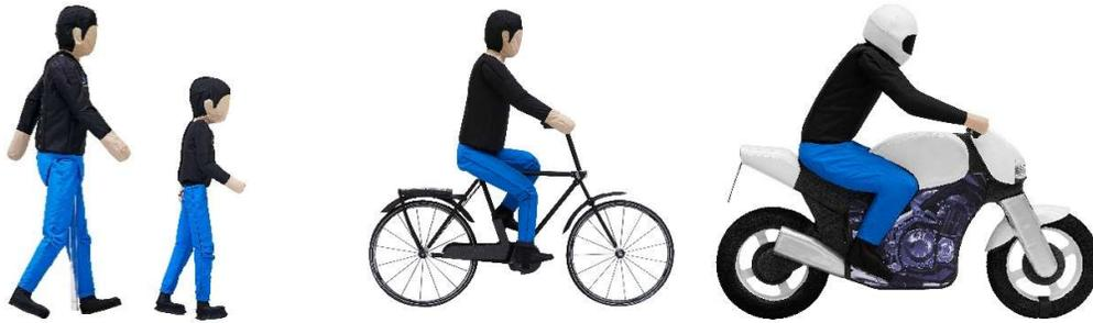
**Figure 5-1: Euro NCAP VRU Targets (EPTa, EPTc, EBTa and EMT)**
