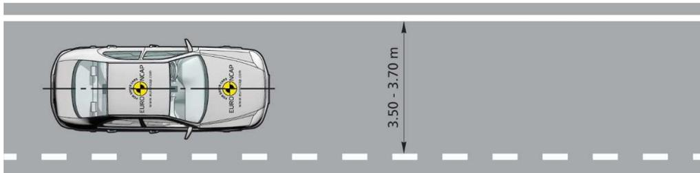
**Figure 6-2: Layout of the lane markings**
