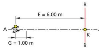
**Figure 7-8 CPTANs scenario – VUT right turn, pedestrian crossing from nearside**
