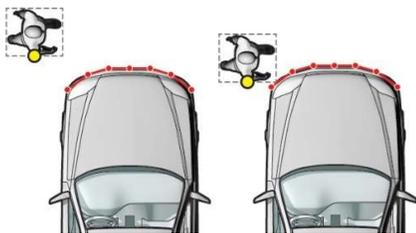
Figure 2-1: Front end profile and EPT
