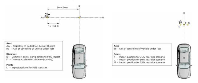
Figure 7-9: CPRA/CPRC scenario, Pedestrian from Nearside (left) and Stationary (right)
