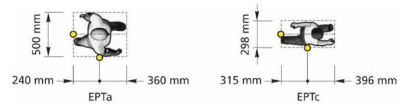
Figure 3-4: Virtual box dimensions around EPTa and EPTc
