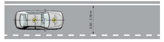
Figure 6-2: Layout of the lane markings
