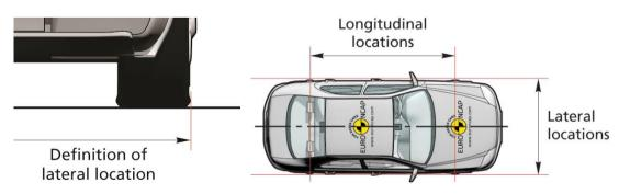
Figure 6-5: Vehicle dimensional measurements
