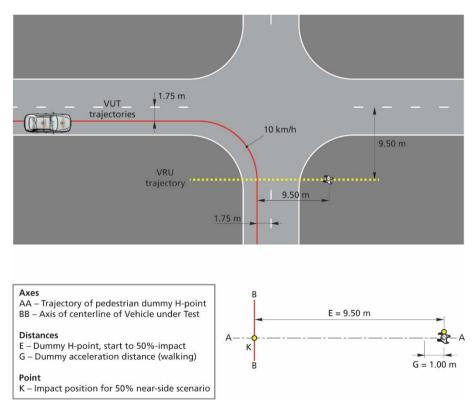
Figure 7-7 CPTAno scenario – VUT right turn, pedestrian crossing from farside
