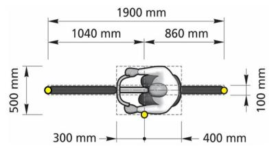
Figure 3-5: Virtual box dimensions around EBT
