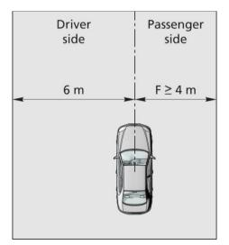
The free space F between the VUT path and the mounting facility shall be  $F \ge 4m$ .
