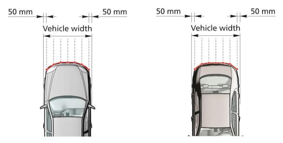
Figure 3-3: Virtual profiled line around both the front end (left) and rear end (right) of the VUT
