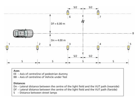
Figure B10: CPFA Night-time setup
