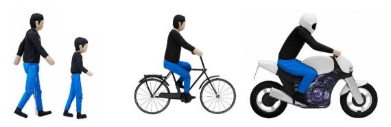
Figure 5-1: Euro NCAP VRU Targets (EPTa, EPTc, EBTa and EMT)
