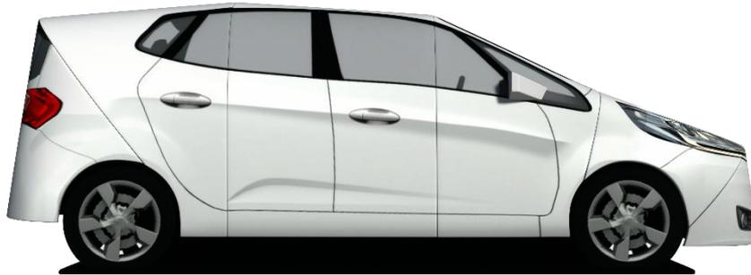
Figure 5-1: Global Vehicle Target (GVT)
