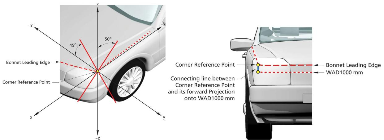
Figure 11: Determination of the corner reference point
