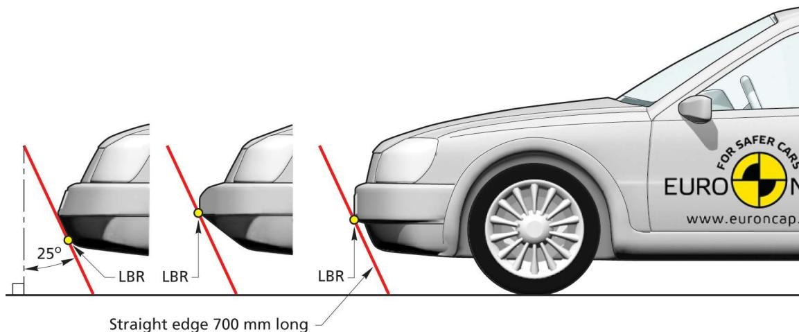
**Figure 13: Determination of the Lower Bumper Reference Line**
