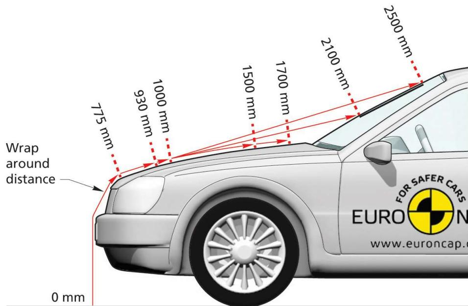
Figure 9: Marking wrap around lines
