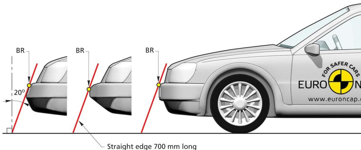
Figure 12: Determination of upper bumper reference line
