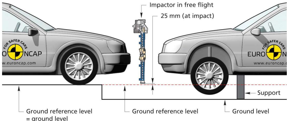
Figure 27: Legform to Bumper tests
