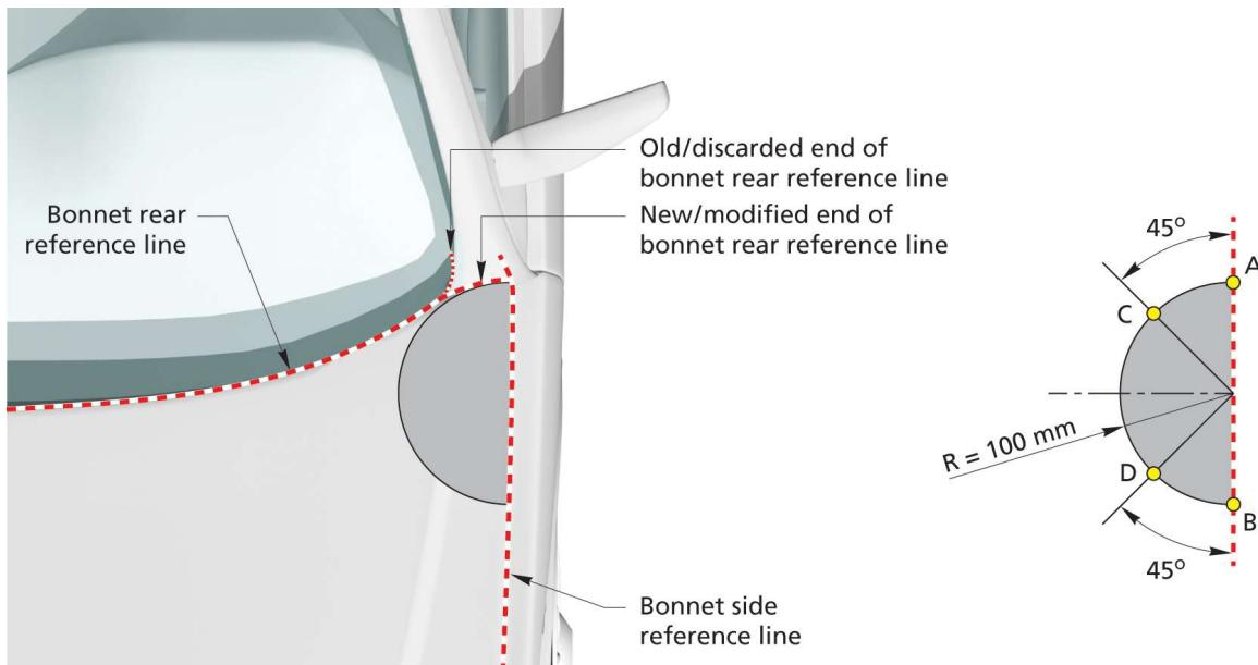
**Figure 8: Bonnet rear reference line template and extension**
