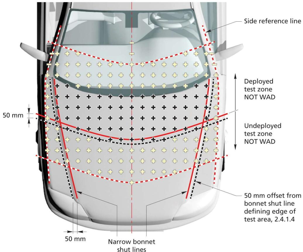
**Figure 2: Area to meet low speed requirements**
