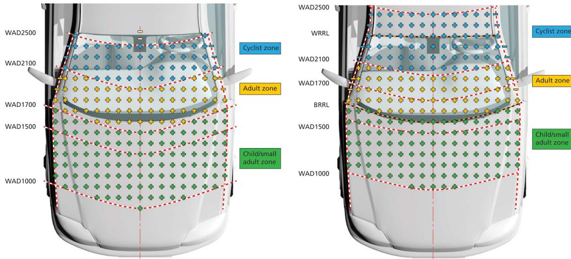
Figure 20 Identification of VRU headform zones
