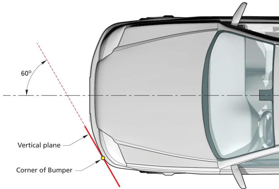
**Figure 14: Determination of bumper corner**
