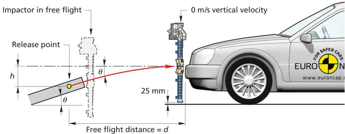
**Figure 29 Ballistic compensation**
