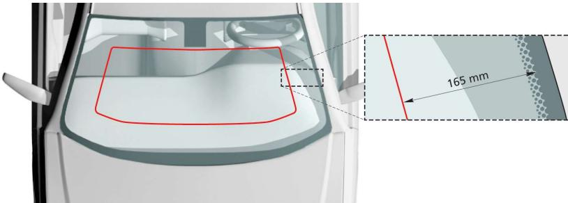
Figure 24: Windspeed periphery measurement
