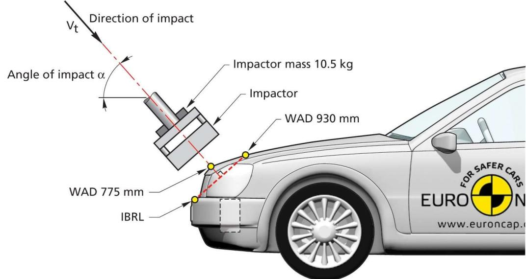
Figure 30: Upper Legform to WAD775mm Test
