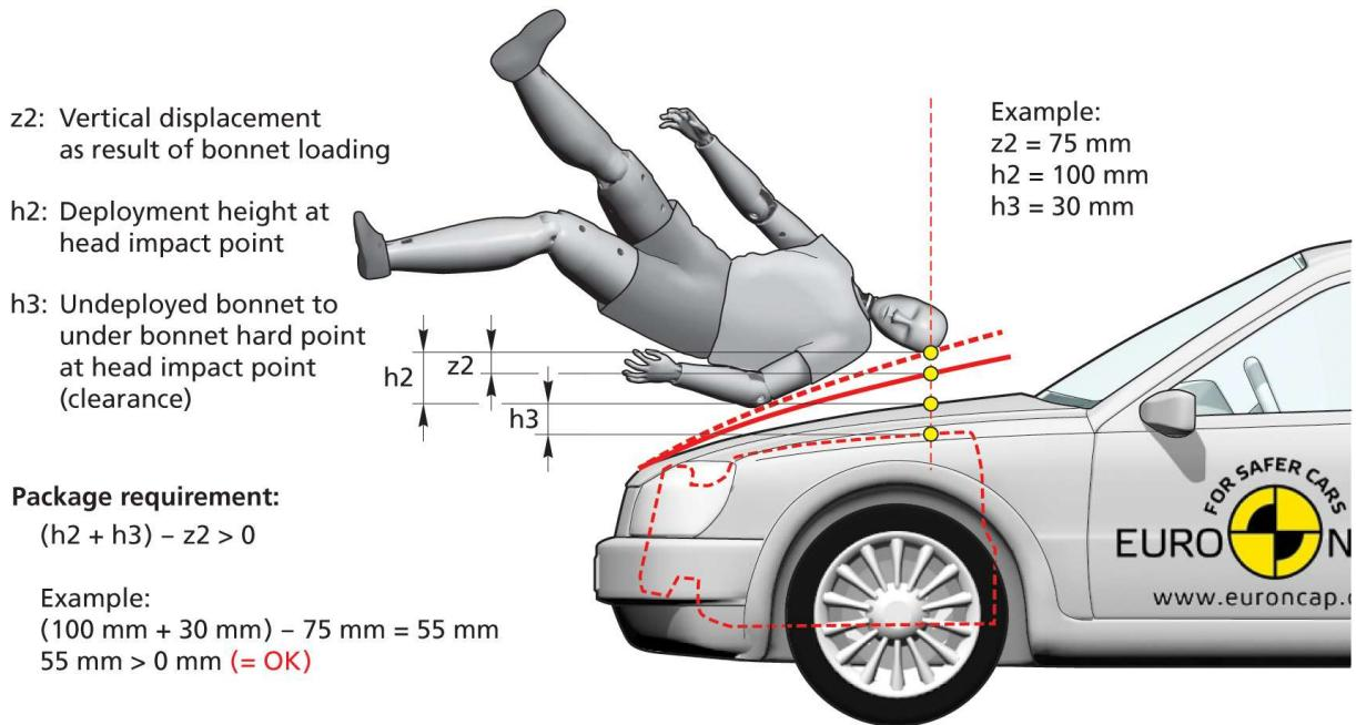
**Figure 4: Bonnet deflection total clearance requirement**
