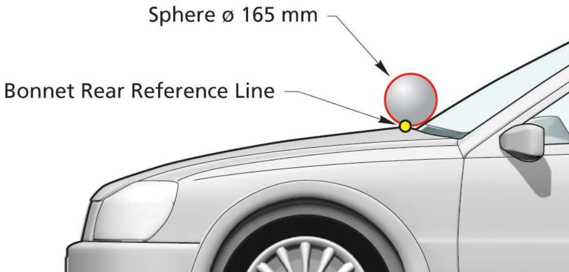
**Figure 7: Determination of the bonnet rear reference line**
