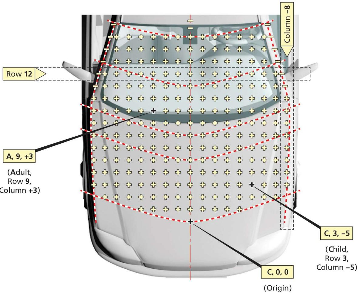
Figure 21 Labelling of the headform grid points
