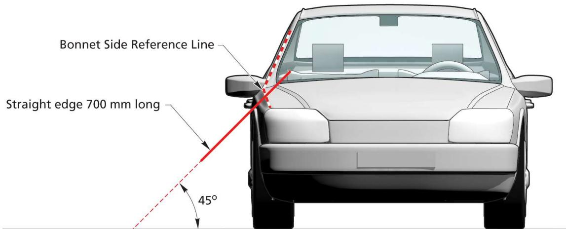
Figure 5: Determination of the bonnet side reference lines
