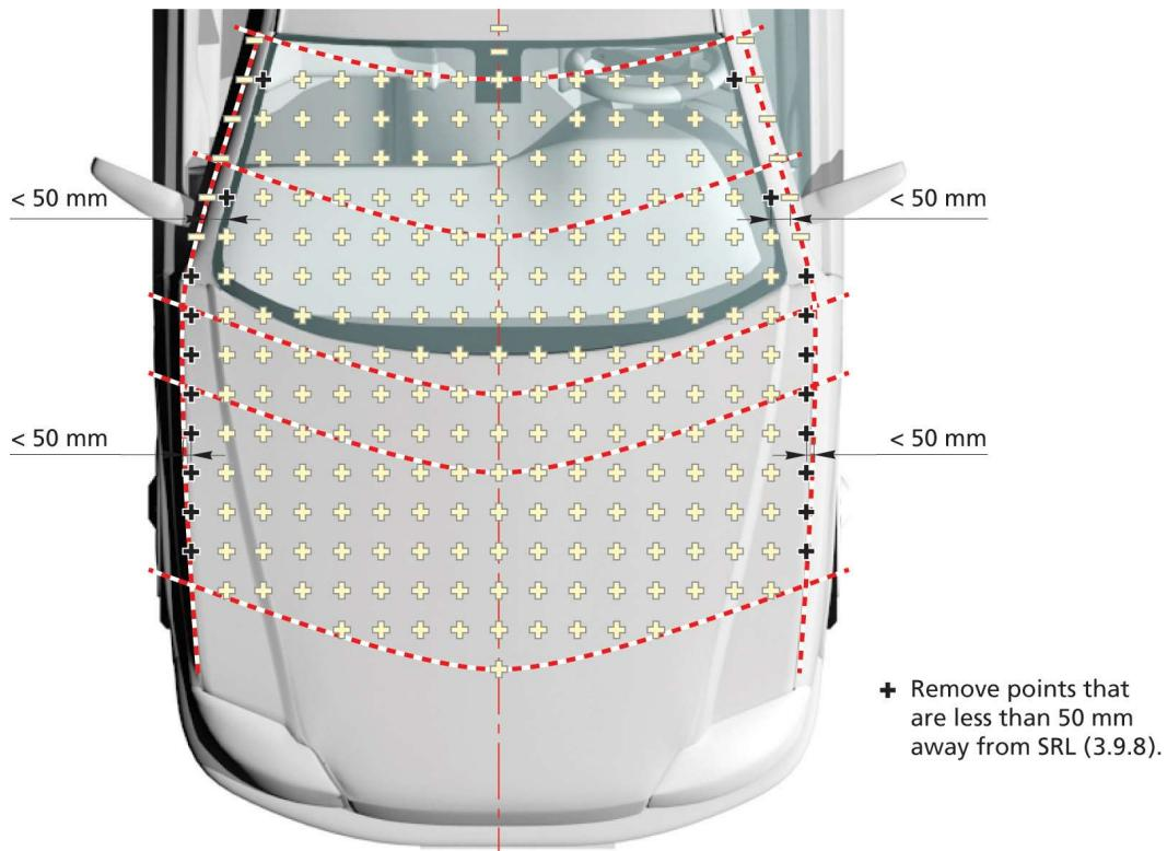
Figure 19: Deleting grid points
