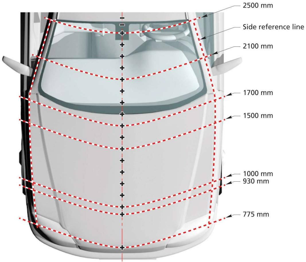
**Figure 10: Headform test area**
